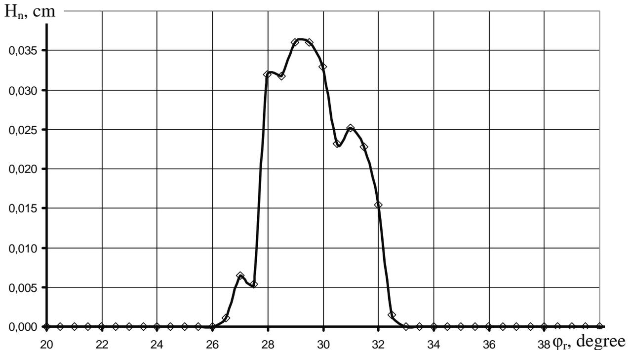
Fig. 4. The dependence of the injector needle height  $H_n$  on the camshaft rotation angle of the pump  $\phi_r$ : high pressure pump 8NK-10;  $n_r = 350 \text{ min}^{-1}$ ;  $Q_c = 190 \text{ mm}^3$
