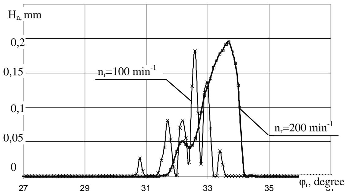
Fig. 2. The dependence of the injector needle height  $H_n$  on the camshaft rotation angle of the pump  $\phi_r$ ; high pressure pump UTN-5;  $Q_c = 72 \text{ mm}^3$
