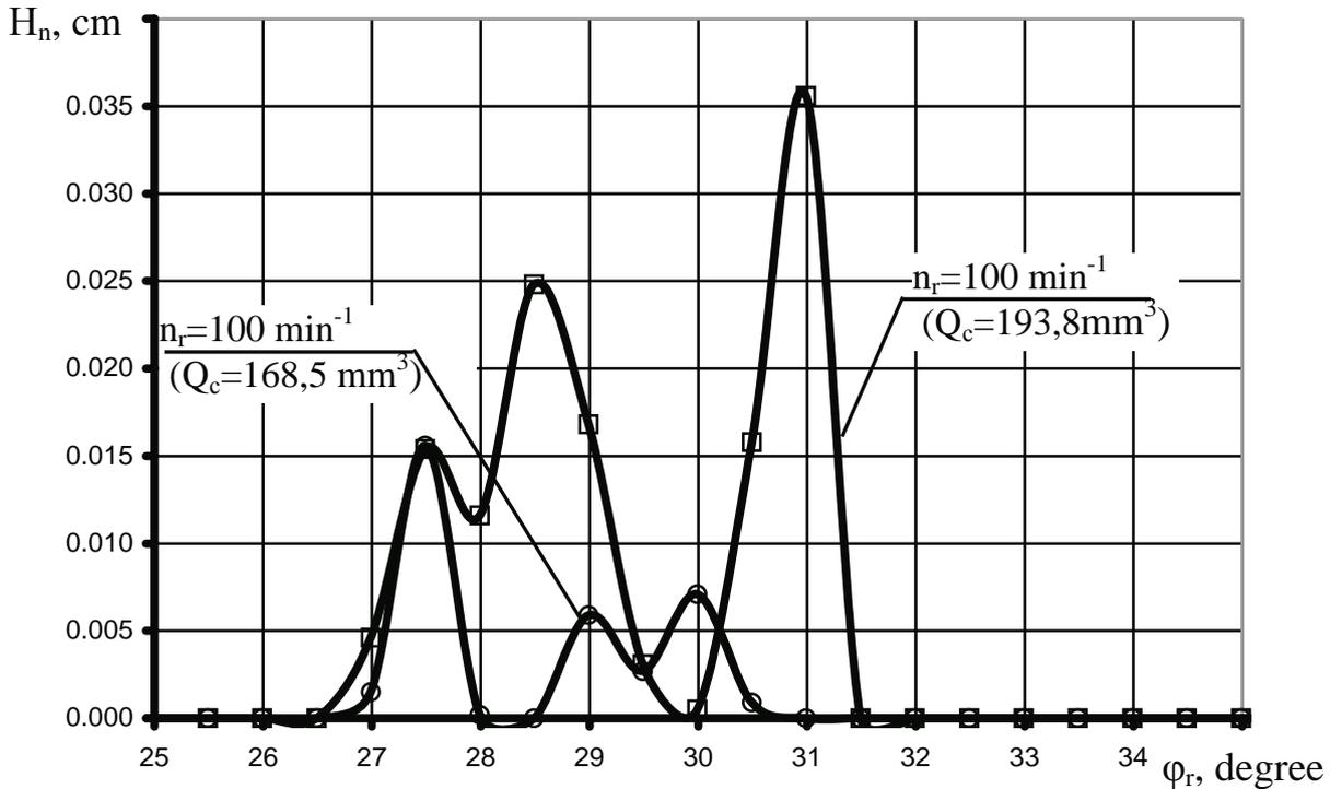
Fig. 3. The dependence of the injector needle rise  $H_n$  on the camshaft rotation angle of the pump  $\phi_r$ : high pressure pump 8NK-10
