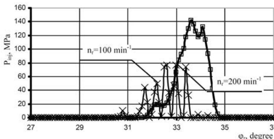
Fig. 1. The dependence of the injection pressure  $P_{inj}$  on the rotation angle of the pump  $\phi_r$ : high pressure pump UTN-5;  $Q_c=72 \text{ mm}^3$
