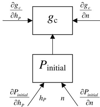
Fig. 5. The structural scheme of interconnection parameters of the fuel feed process for functional dependencies:
